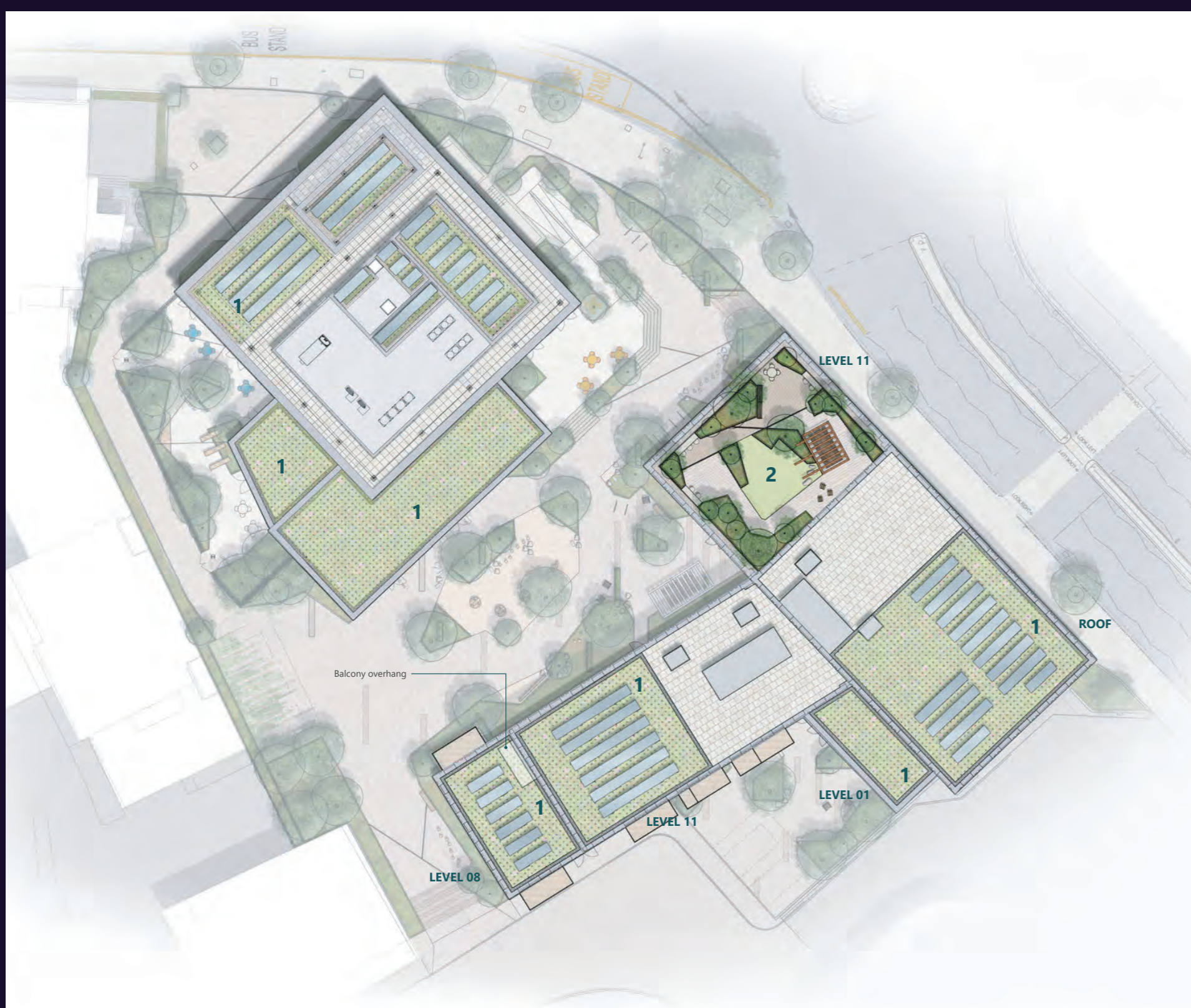
Green roofs and roof terrace
